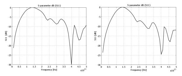
**Fig. 2:** Frequency response of reflection coefficient in range from 1 to 50 GHz. Left:  $\lambda_{\epsilon}/2$ , normal mesh (6 708 DOF, 164 s). Right:  $\lambda_{\epsilon}/2$ , finer mesh (36 789 DOF, 3 437 s).
