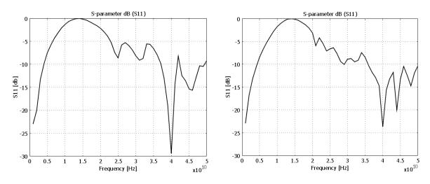
Fig. 3: Frequency response of reflection coefficient in range from 1 to 50 GHz if PBC are used. Left: λ<sub>∈</sub>/2, normal mesh (7 481 DOF, 295 s). Right: λ<sub>∈</sub> (25 401 DOF, 2 427 s).
